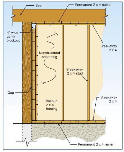
Recommended breakaway wall construction.
