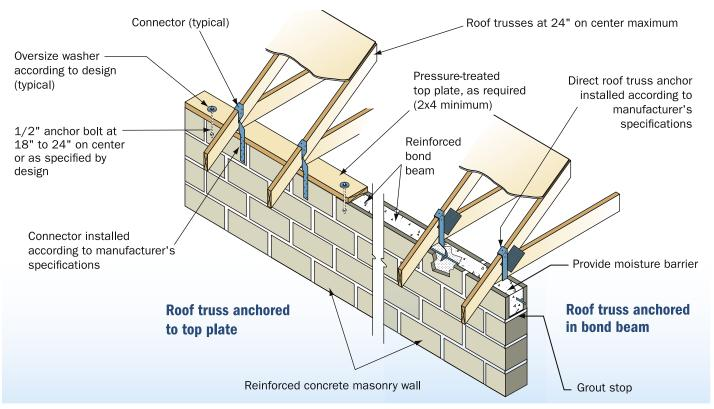
Roof framing to masonry wall.
