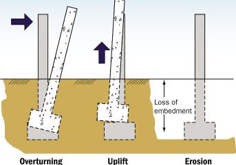
Piers are subject to upward, downward, and horizontal loads. Pier reinforcement and footing size are critical to resisting these loads; therefore, pier and footing design must be verified by an engineer.
