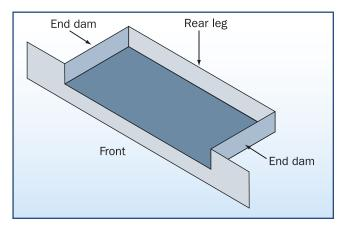
Figure 1 Pan flashing.
