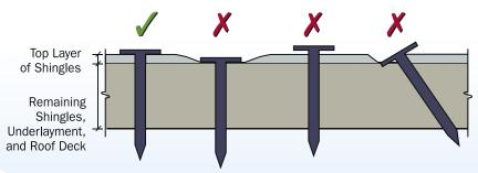
"The Good, the bad, and the ugly" - Properly driving roofing nails.
