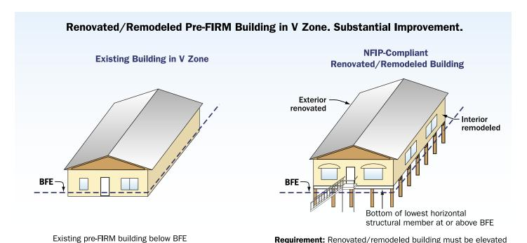
Figure 2 Substantial improvement: Renovated/remodeled building in a V zone.
