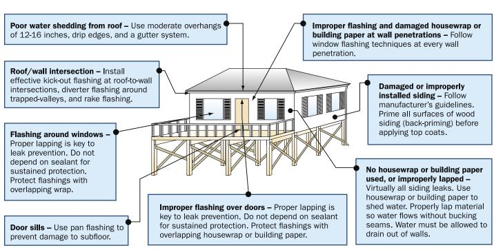
The location of water entry is often difficult to see, and the damage to substrate and structural members behind the exterior wall cladding frequently cannot be detected by visual inspection.
