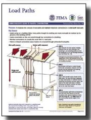
Fact Sheet No. 10, Load Paths – Illustrates the concept of load paths and highlights important connections in a typical wind uplift load path.
