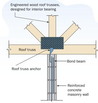
Roof framing to interior masonry wall
