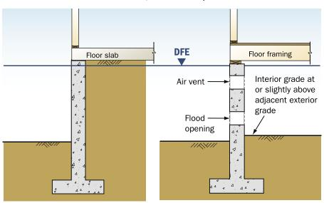
Floor slab atop backfilled stemwall foundation
