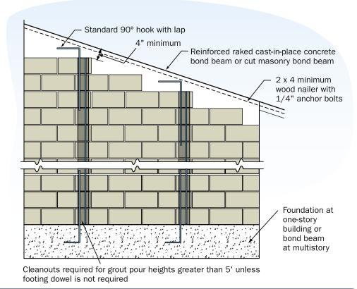
Continuous gable endwall reinforcement.
