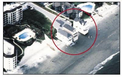
Figure 1. Well-built but poorly sited building.
