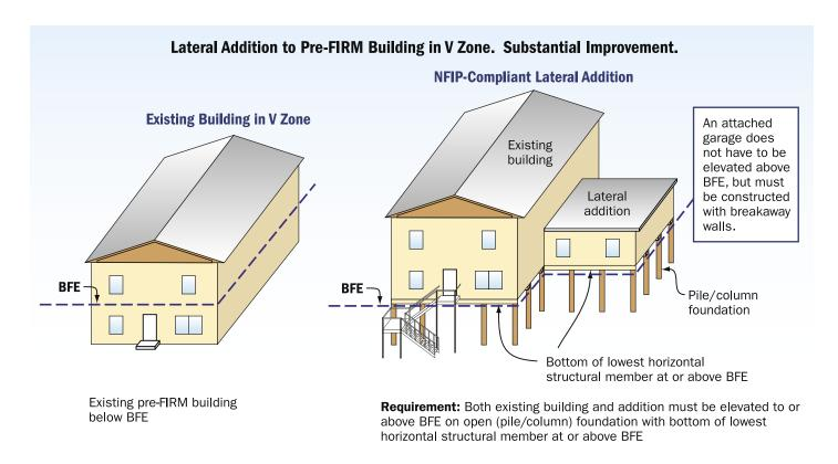
Figure 3 Substantial improvement: Lateral addition to a pre-FIRM building in a V zone.
