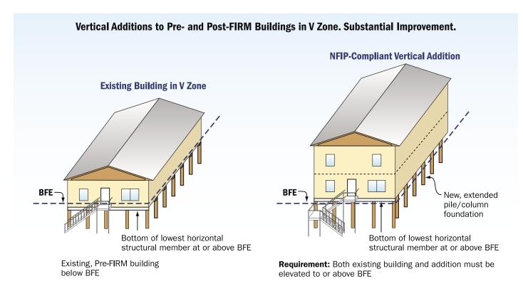
Figure 5 Substantial improvement: Vertical addition to a pre-FIRM building in a V zone.
