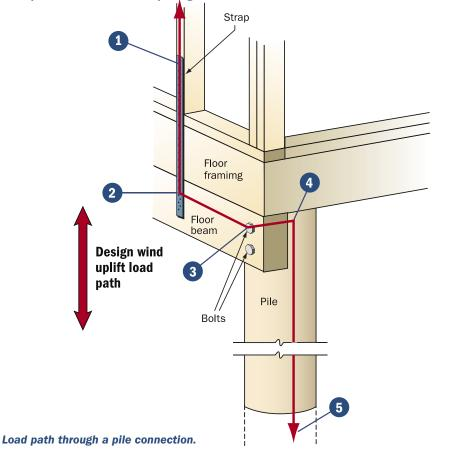
Load paths can be complex through a connection. It is important that each link within the connection be strong enough to transfer the full design load.
