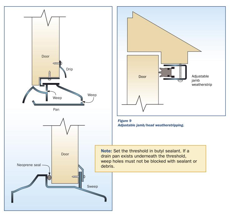
Figure 8 Thresholds.
