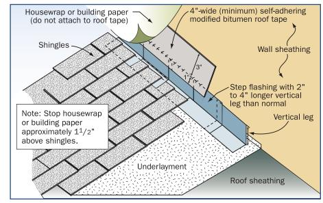
Figure 1 Roof/wall flashing detail.
