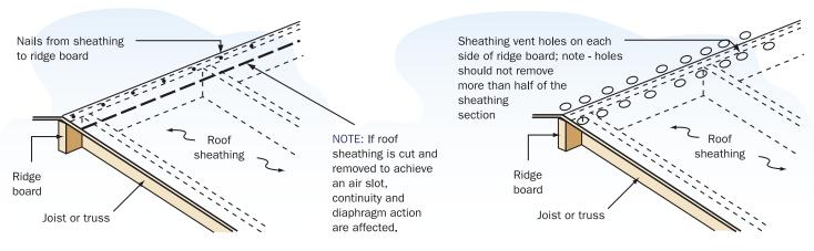
Method for maintaining a continuous load path at the roof ridge by nailing roof sheathing.
